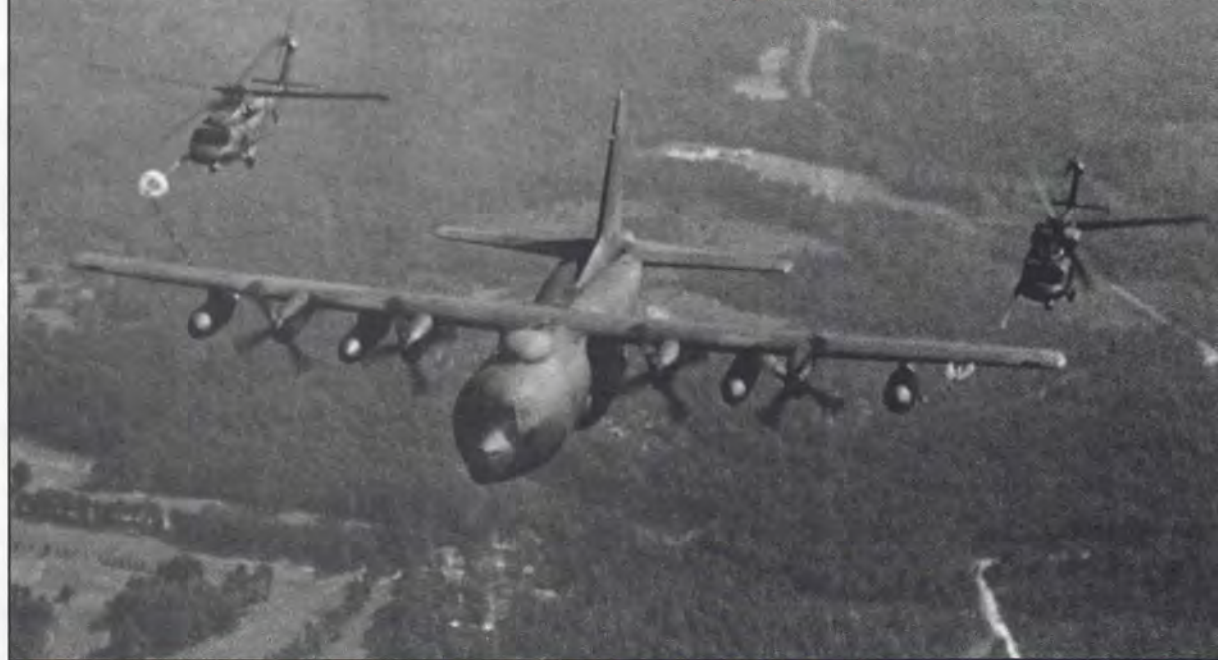
An MH-60G Pave Hawk ( right ) nudges its aerial refueling probe toward the drogue of a HC-130 Combat Shadow as a sister ship takes on fuel.
